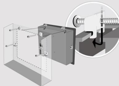
Plan for adequate space around the unit and inside the enclosure, for ventilation and cables. Consider the heat from other devices inside the enclosure. The ambient temperature around the unit must be 0 ~ 50°C
