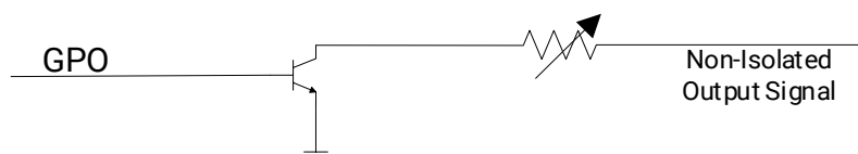
Figure 5-3 Internal Circuit of Output Signal
