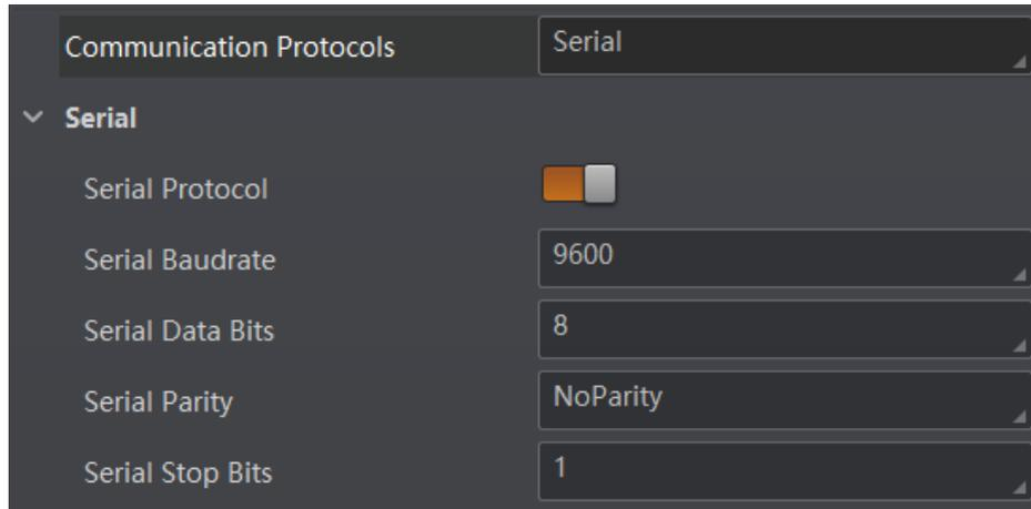
The screenshot shows a configuration window with a dark background. At the top, 'Communication Protocols' is set to 'Serial'. Below this, a section titled 'Serial' is expanded. It contains five settings: 'Serial Protocol' is a toggle switch that is turned on (orange); 'Serial Baudrate' is a text input field containing '9600'; 'Serial Data Bits' is a dropdown menu set to '8'; 'Serial Parity' is a dropdown menu set to 'NoParity'; and 'Serial Stop Bits' is a dropdown menu set to '1'.
