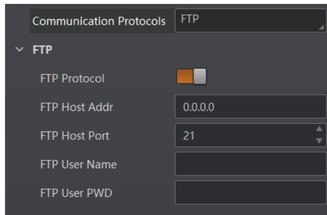
The screenshot shows a configuration window with a dark background. At the top, 'Communication Protocols' is set to 'FTP'. Below this, a section titled 'FTP' is expanded. It contains five settings: 'FTP Protocol' is a toggle switch that is turned on (orange); 'FTP Host Addr' is a text input field containing '0.0.0.0'; 'FTP Host Port' is a spinner control set to '21'; 'FTP User Name' is an empty text input field; and 'FTP User PWD' is an empty text input field.
