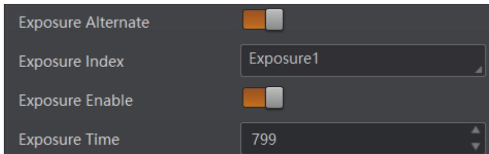
Figure 8-3 Alternate Exposure
