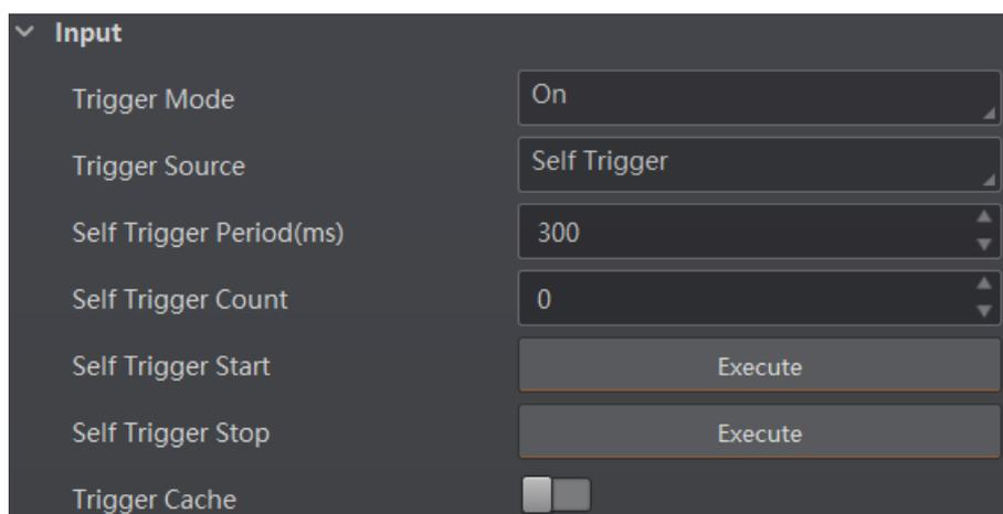
Figure 8-30 Set and Execute Self Trigger Mode
