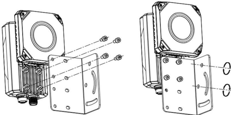
**Figure 4-2 Front Installation**
