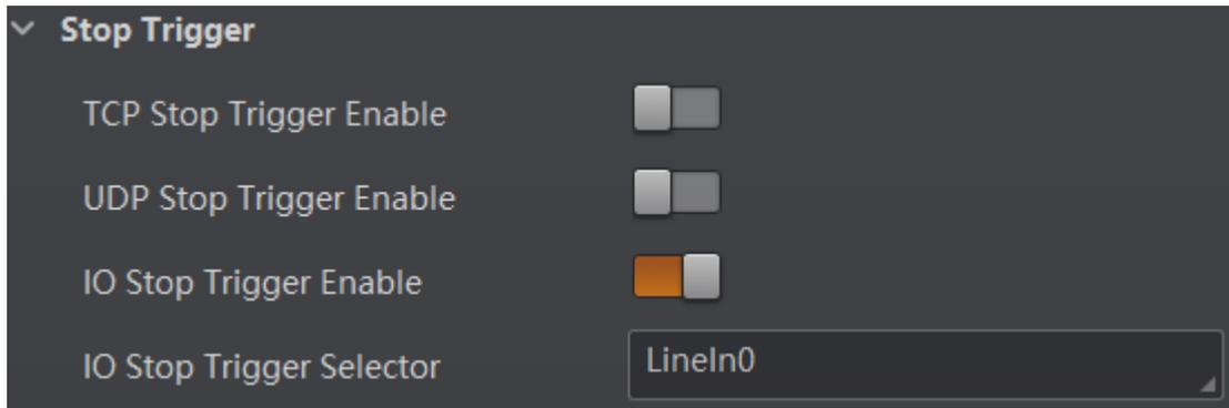
Figure 8-33 IO Stop Trigger
