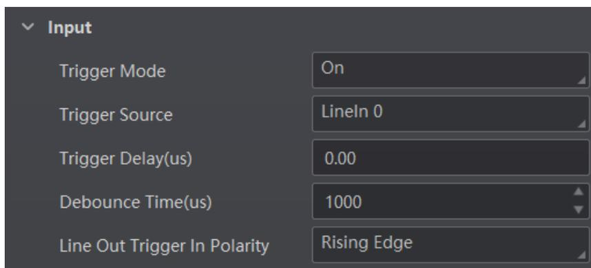
Figure 8-25 Set and Execute Hardware Trigger Mode
