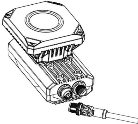
**Figure 4-3 Gigabit Ethernet Interface Wiring**
