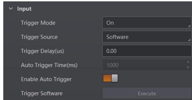
Figure 8-24 Set and Execute Software Trigger Mode
