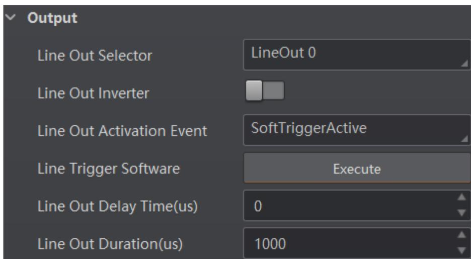
Figure 8-46 Select Soft Trigger Active
