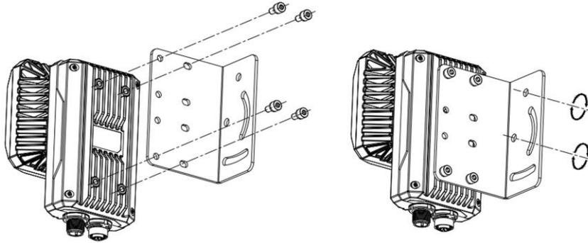
**Figure 4-1 Rear Installation**
