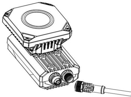
**Figure 4-4 Power and I/O Wiring**
