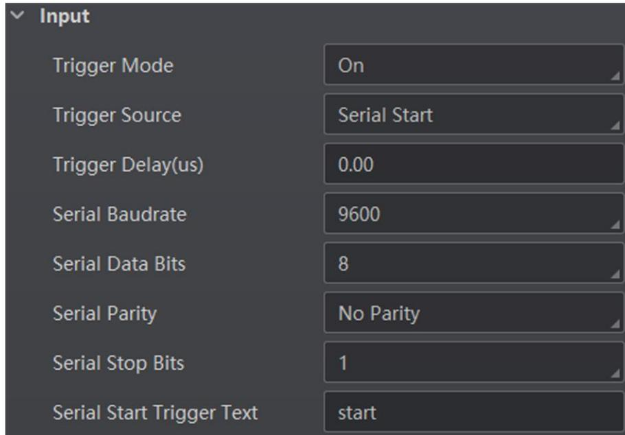
Figure 8-29 Set and Execute Serial Port Trigger Mode
