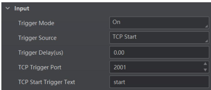
Figure 8-27 Set and Execute TCP Trigger Mode
