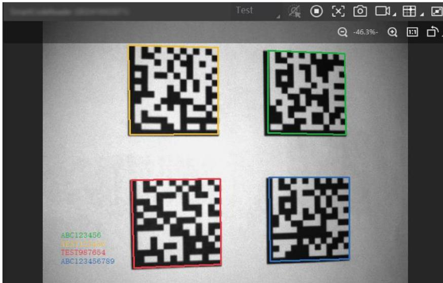
**Figure 7-2 Code Reading**
