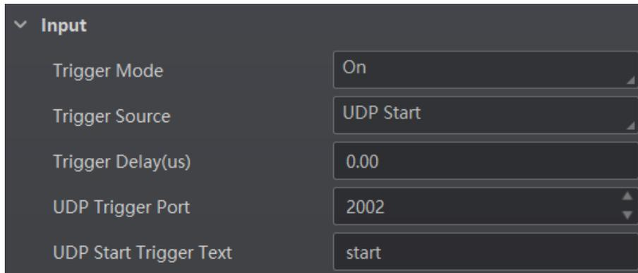
**Figure 8-28 Set and Execute UDP Trigger Mode**
