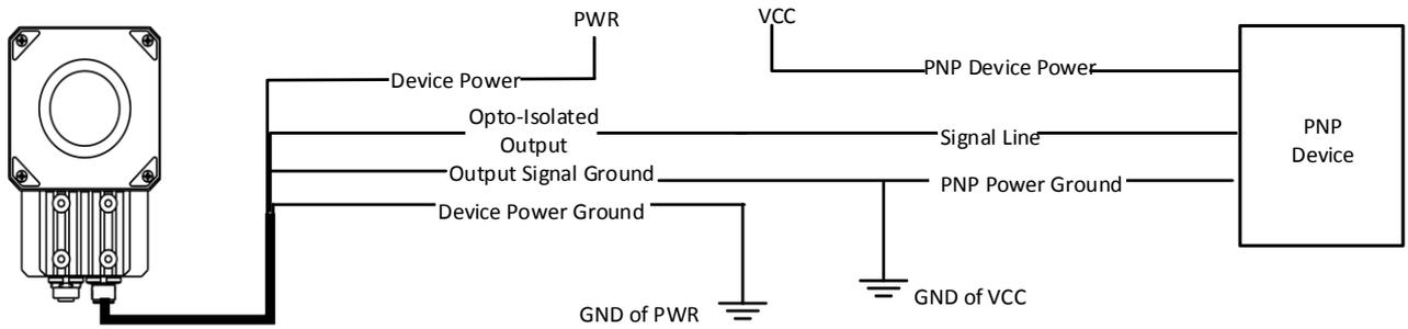
**Figure 3-8 Output Signal Connecting to PNP Device**
