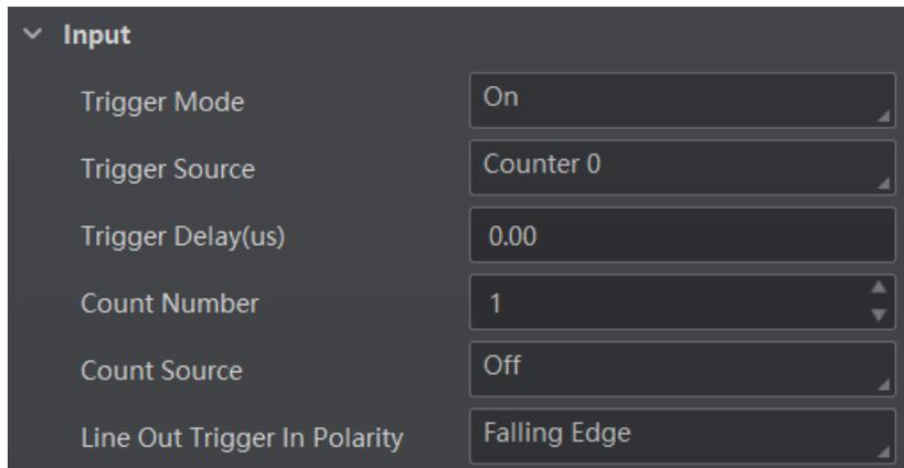
Figure 8-26 Set and Execute Counter Trigger Mode
