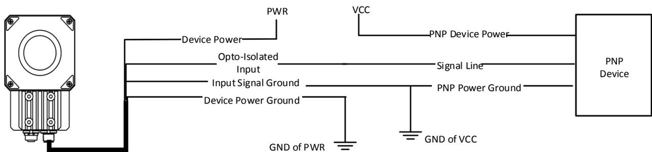
**Figure 3-5 Input Signal Connecting to PNP Device**
