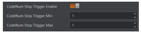
Figure 6-51 Stop Trigger via Code Number
