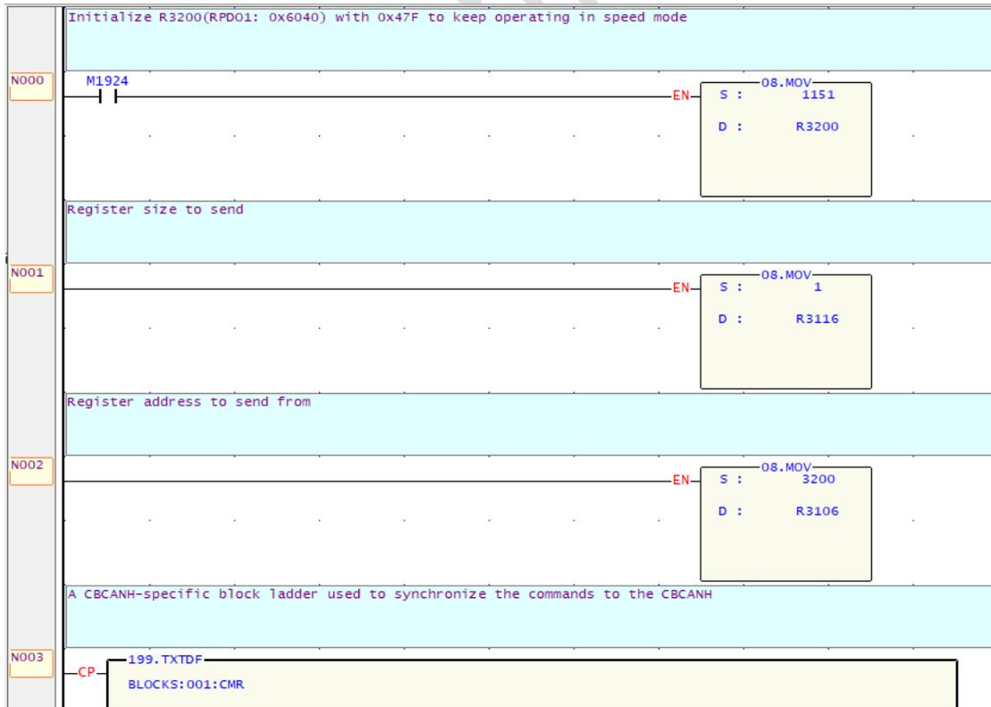
**Figure 21 Example program for turning on a motor**
