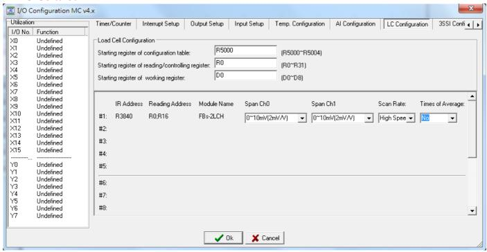
Before FBs-2LCH module can be working, the configuration of the module should be set by the Winproladder software tool. The picture shown at above is the I/O configuration page for "LC module" setup.
