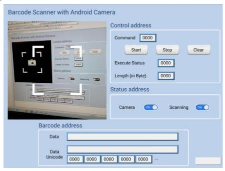
3. When a QR code is read, the Execute Status turns 1, and the QR code is captured, its content will be displayed in Barcode Address group box. Unicode is also supported.
