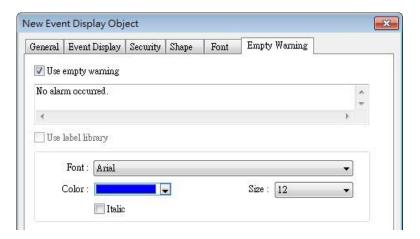
When [Use empty warning] is enabled, the text displayed when no event has occurred can be specified. This feature is not supported on cMT / cMT X Series models.
