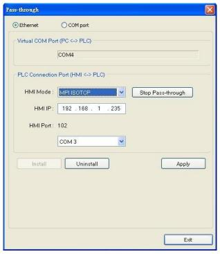
2. In STEP 7, go to [Option] » [Set PG/PC Interface]. Confirm that the interface used is "PC Adapter(MPI)", and then click [Properties]. Select the same COM port as the virtual serial port. In the example COM 4 is used.
